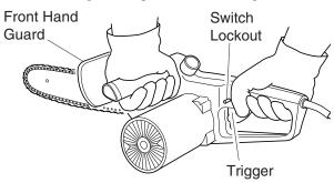
Figure 9 - Front Hand Guard, Switch Lockout, and Trigger Location
